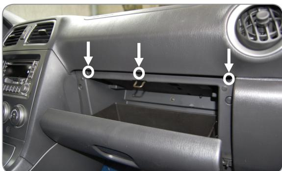
**EN** Remove the glove compartment
