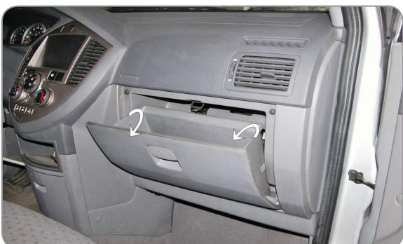
**(EN)** Remove the glove compartment
