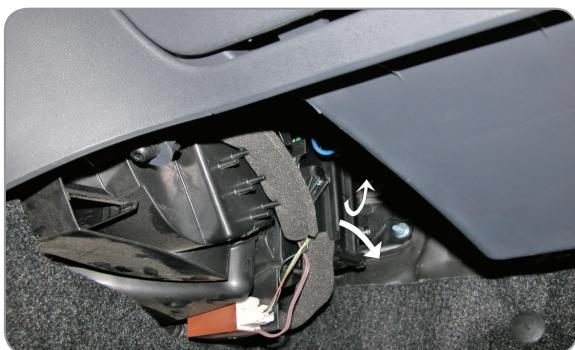
EN Open the filter chamber, gently remove the old filter, put in the new one and carry out the opposite to all the previously mentioned operations in the reversed order
