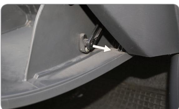
**(EN)** Remove the glove compartment
