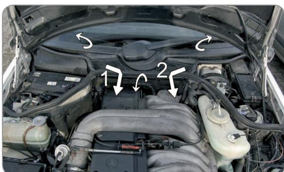
EN Remove the rubber seal. Remove the first section of the screen. Remove the second section of the screen
