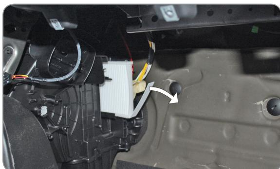
EN Carefully remove the first filter
