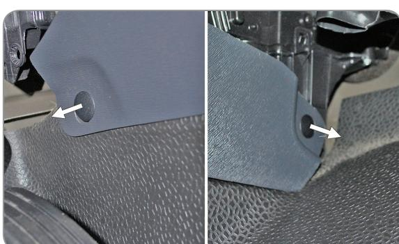
**(EN)** Remove the protecting device
