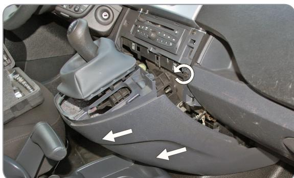
(EN) Remove the element shown in the picture. Loosen the screw
