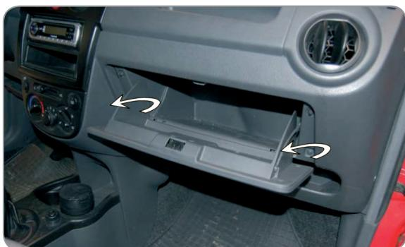
**(EN)** Filter is located behind the glove compartment. Loosen the screws and remove the upper wall of the locker
