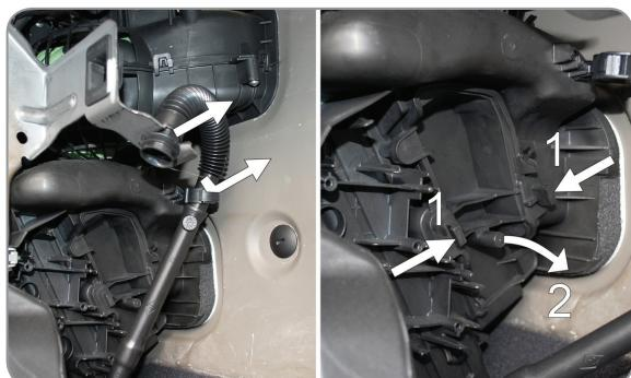
**EN** Disassemble the segment of the ventilation collector pipe and remove the collector. Remove the housing
