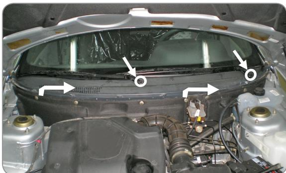
**(EN)** Unscrew the wipers. Remove the rubber seal
