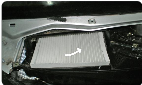
**(EN)** Gently remove the old filter, put in the new one and carry out the opposite to all the previously mentioned operations in the reversed order
