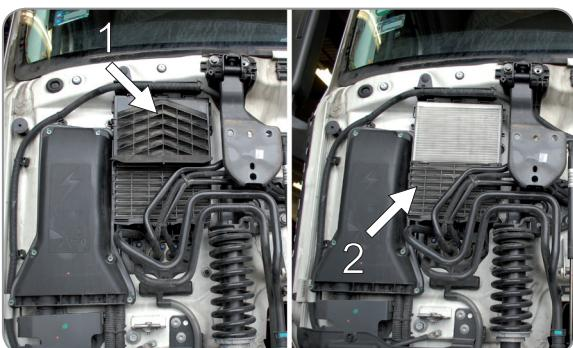
**(EN)** Remove the filter housing
